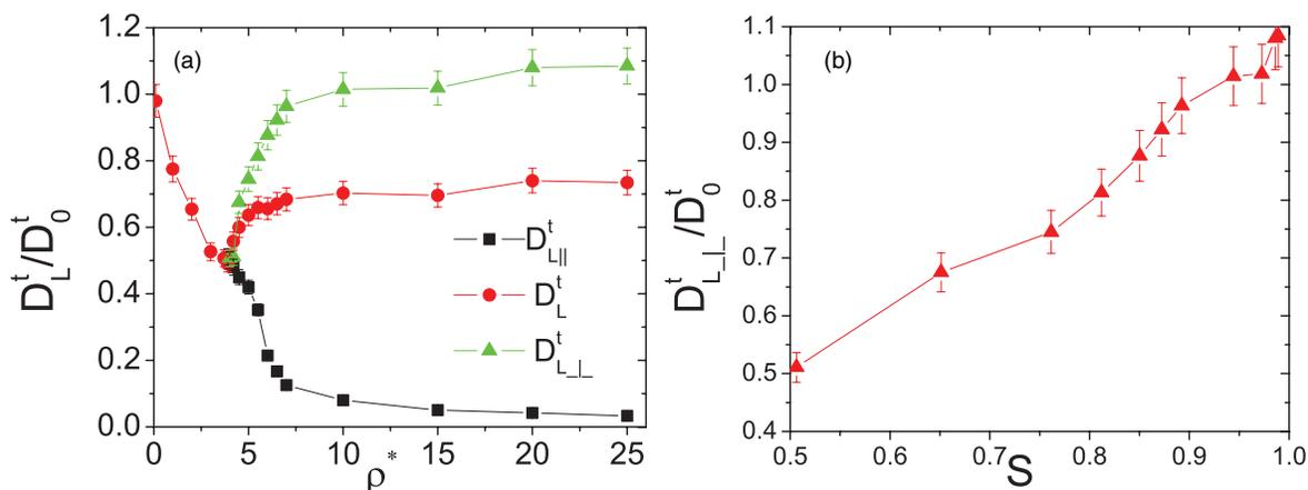
FIG. 7. (a) Long-time average diffusion coefficient  $D_L^t$  (in both isotropic and nematic phases) and long-time diffusion coefficients in directions parallel  $D_{L\parallel}^t$  and perpendicular  $D_{L\perp}^t$  to the nematic director for densities  $\rho^* \geq 4$ . (b)  $D_{L\perp}^t$  as a function of nematic order parameter.
