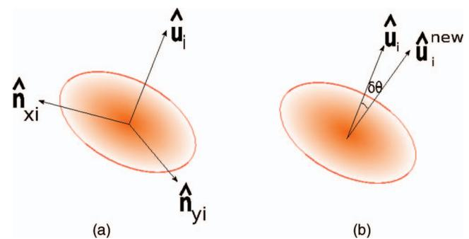
FIG. 1. A schematic drawing presenting (a) an example of an axially symmetric object with its orientation vector  $\hat{u}_i$  together with its body frame defined by  $\hat{u}_i$  and two mutually perpendicular vectors  $\hat{n}_{xi}$  and  $\hat{n}_{yi}$ . (b) Rotation of orientation vector with an angle  $\delta\theta$ .
