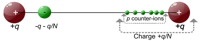
FIG. 3. (Color online) Upon regrouping the p + 1 leftmost counterions in Fig. 1, one obtains an ion with charge -q - q/N . This newly defined system has the same large distance pressure as that of Fig. 1.
