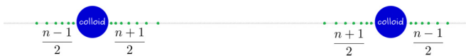
FIG. 3. Fundamental configuration for P = 0 and N = 2n = 26 (even) and n = 13 (odd). In this case, the first threshold is precisely P_0 = 0 . As soon as P increases and 0 < P \leq P_1 , one particle from each interior side will go to the outside, leaving (n - 1)/2 particles in each interior side of the colloid and (n + 1)/2 on each outer side.
