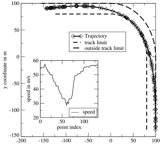
**Figure 2.** The trajectory and speed of a vehicle in a curve obtained after heuristical optimization with the Metropolis algorithm.
