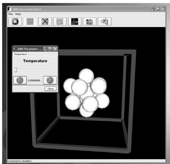
**Figure 1.** A screenshot of the JIMD visualization program interacting with the Metropolis simulation of a LJ13 cluster: the temperature can be interactively changed.
